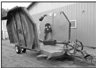
Woods 3240 , batwing mower, 20' cut, large 1000 PTO, chain guards, 28x7.7-14 airplane tires, stored inside . . . . . $13,900
